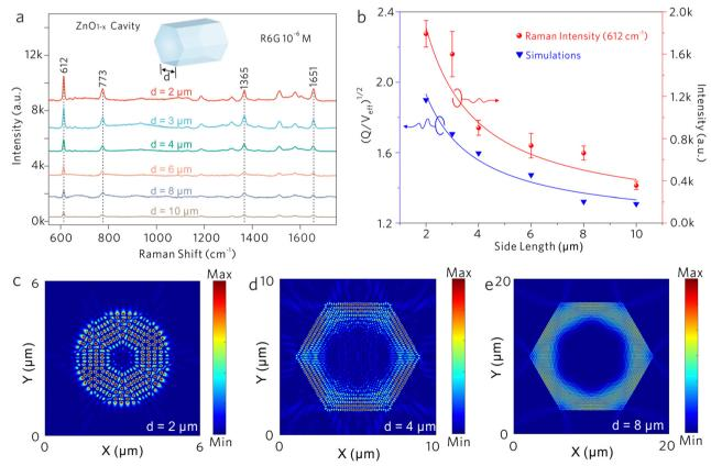
Fig. 5 WGM cavity sensing mechanisms: Purcell effect. (a) Raman spectra of R6G molecules acquired on  $ZnO_{1-x}$  cavities with different d values. (b) The relationships of Raman intensities versus side length, and the  $(Q/V_{eff})^{1/2}$  values versus the side length. Electrical field distribution of the fundamental mode in the X-Y plane from different  $ZnO_{1-x}$  cavities: (c)  $d=2 \mu m$ , (d)  $d=4 \mu m$ , and (e)  $d=8 \mu m$ .
