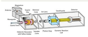
Fig. 1 Schematic depiction of the MICAP-MS.
