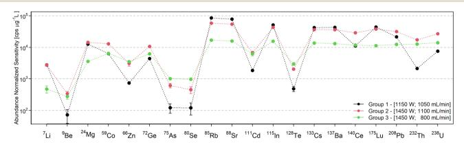
Fig. 4 Response curves of the optimal plasma operating conditions according to the three types of sensitivity behaviours seen in the contour plots. Measurements were performed with the standard interface & pump configuration. The operating conditions corresponding to the three analyte groups are given. The error bars represent two times the standard deviation and are only visible for some elements. (All lines are to guide the eye.)
