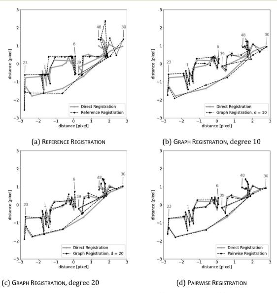
Fig. 6 Registration results on the twig dataset with the element potassium using (a) reference registration, (b) graph registration with d = 10, (c) graph registration with d = 20, and (d) pairwise registration. The result of direct registration is shown as a reference in every image.
