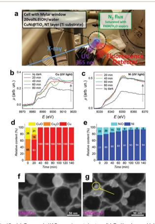
Fig. 13 (a) Operando XAS experimental setup; (b) Cu K-edge and (c) Ni K-edge XAS spectra of 5Ni5Cu-TiO2 in a water-ethanol under UV irradiation for various exposure times; (d) Cu and (e) Ni phase contents determined by operando XAS for 5Ni5Cu-TiO2; SEM images of 5Ni5Cu-TiO<sub>2</sub> (f) before and (g) after photocatalysis (a yellow circle indicates metallic NPs deposited under the UV irradiation). Adapted with permission from ref. 171; copyright 2020 ACS.
