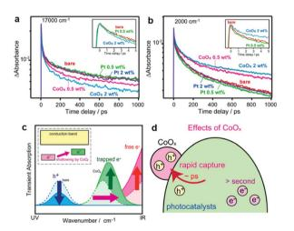
Fig. 10 Decay of transient absorption at (a) 17 000 cm<sup>-1</sup> and (b) 2000 cm<sup>-1</sup> for bare, CoO<sub>x</sub>-loaded, and Pt-loaded LaTiO<sub>2</sub>N after excited by 500 nm laser pulses; (c and d) schematics showing the change in carrier dynamics upon  $CoO_x\ CC$  loading. Adapted with permission from ref. 157; copyright 2014 ACS
