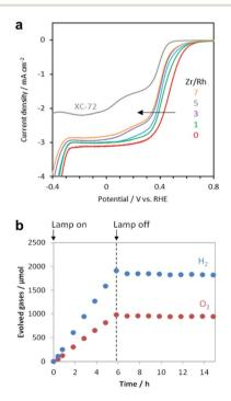
Fig. 12 (a) Current-potential curves of RhZrO<sub>x</sub> (Zr/Rh: 0-7 w/w)loaded carbon supports in O<sub>2</sub>-saturated 1 M Na<sub>2</sub>SO<sub>4</sub> (pH 7); (b) gas evolution over time by  $RhZrO_x/SrTiO_3$ :Al (Rh = 0.1 wt% and Zr = 0.5 wt% vs. SrTiO<sub>3</sub>: Al) during and after light irradiation (300 W Xe lamp). Adapted with permission from ref. 169; copyright 2020 RSC.
