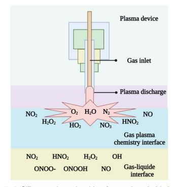
Fig. 3 Different reactive species originate from gas plasma, both in the atmosphere and at the gas-liquid interfaces.
