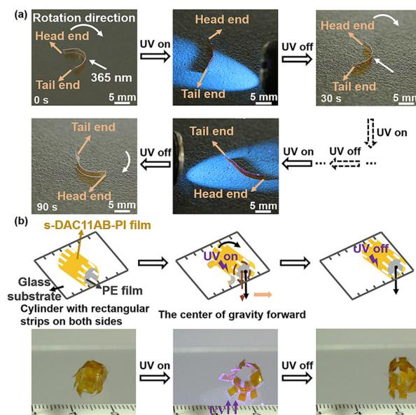
**Fig. 4** (a) The rotating robot prepared using the s-DAC11AB-PI/PE film, which rotates on a rough surface under UV light irradiation. (b) Photographs of the rolling motion enabled by UV light irradiation from the underside of the glass substrate. UV light:  $365\ \text{nm}$ ,  $70\ \text{mW cm}^{-2}$ .
