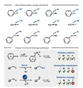
Fig. 1 Top: Bond dissociation energies for aromatic and aliphatic C-X bonds.4 Bottom: Oxidative addition, nucleophilic substitution, and reductive cleavage of C-X bonds.
