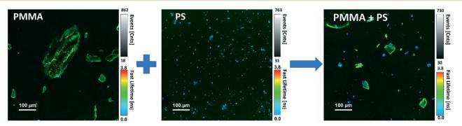
Fig. 3 FLIM microscopy images of PMMA and PS MNPs labelled with HA-RB, before and after mixing the two samples.
