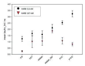
Fig. 4 Mean values with standard deviations of "\(\tau\_\text{Av\_Int"}\), i.e., the average lifetime weighted on intensity, for MNP samples incubated with 170 nM HA-RB (red triangles) and 5.6 nM HA-RB (black circles).
