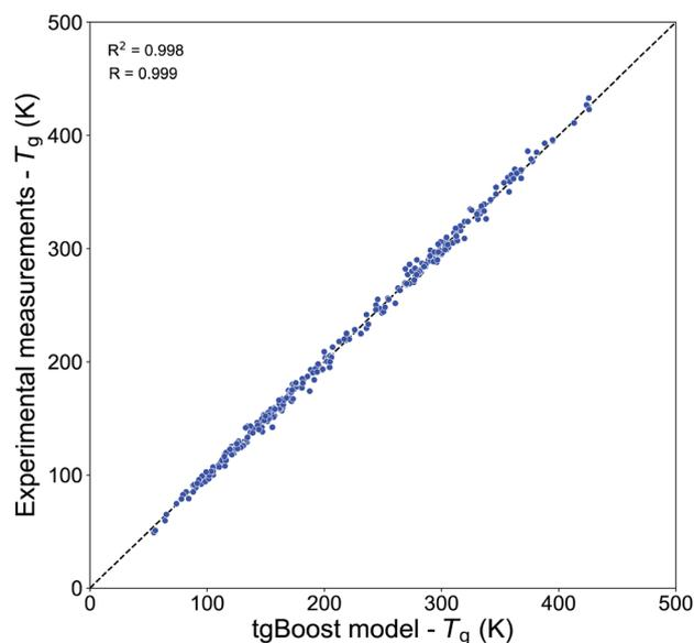
Fig. 2 Correlation plot between the predicted  $T_g$  values by the tgBoost model and the experimental  $T_g$  values from the  $T_g$ -Measured dataset.
