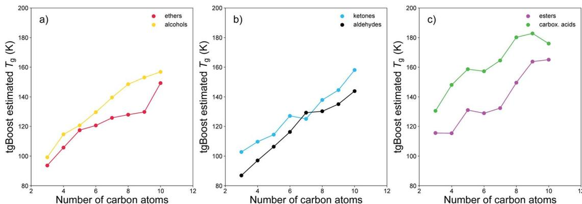
Fig. 6 Estimated  $T_g$  of weakly functionalized isomeric molecules by functional group as a function of the number of carbon atom within the molecule. Isomers are grouped as (a) ethers and alcohols, (b) ketones and aldehydes, and (c) esters and carboxylic acids. The respective functional groups are positioned at the end of the alkyl chain for all species.
