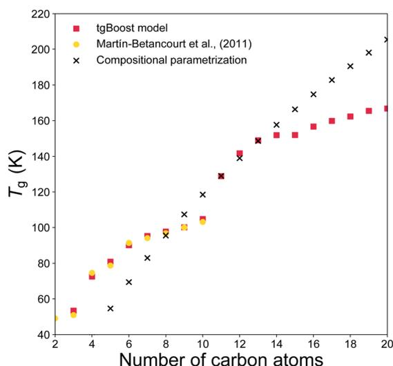
Fig. 3  $T_g$  values predicted for the  $n$ -alkanes ( $n = 2$ –20) by the developed tgBoost model (red dots), molecular dynamics simulations (yellow squares),<sup>38</sup> the  $T_g$  compositional parameterizations (black crosses).<sup>8</sup>
