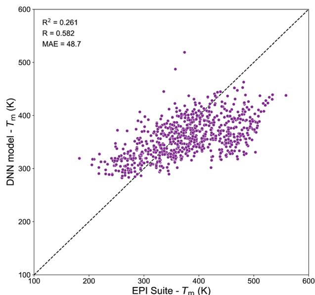
Fig. 9 Correlation plot between the  $T_m$  values predicted by the DNN model and by the MPBPWIN module of EPI Suite for SOA compounds from Shiraiwa *et al.*<sup>56</sup>
