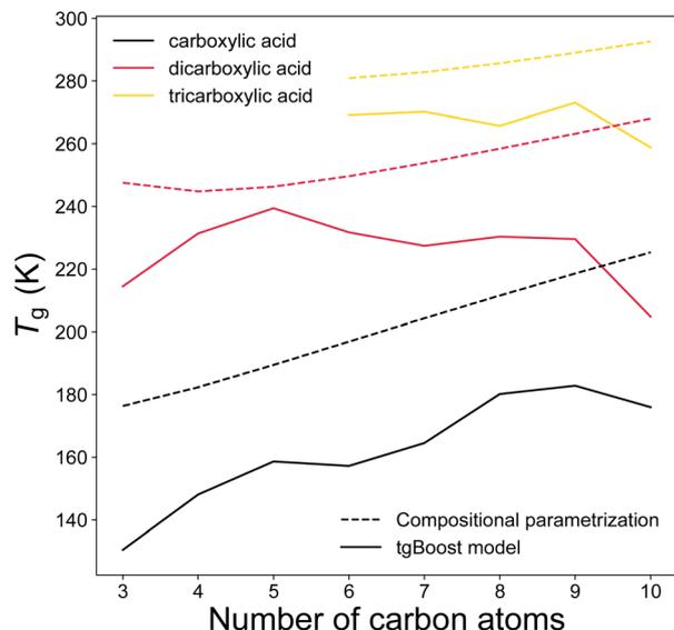
Fig. 7  $T_g$  of linear monocarboxylic, dicarboxylic and tricarboxylic acids as a function of the number of carbon atoms in the alkyl chain as predicted by the tgBoost model (solid lines) and the  $T_g$  compositional parametrization (dashed lines).<sup>8</sup>
