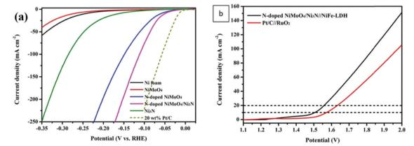
Fig. 115 Polarisation curves of Ni foam, NiMoO<sub>4</sub>, N-doped NiMoO<sub>4</sub>, Ni<sub>3</sub>N and N-doped NiMoO<sub>4</sub>/Ni<sub>3</sub>N heterostructure (a). LSV curves of N-doped NiMoO<sub>4</sub>/Ni<sub>3</sub>N//NiFe-LDH and commercial Pt/C//RuO<sub>2</sub> systems in 1.0 M KOH solution without iR correction (b). Reproduced with permission from ref. 1457. Copyright American Chemical Society 2020
