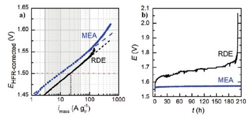
Fig. 144 Evaluation of the OER (a) activity and (b) stability versus time at a given representative OER current in MEA (blue) and RDE (black) configuration for a state-of-the-art commercial IrO2 catalyst. Reproduced from ref. 20 with permission from Wiley
