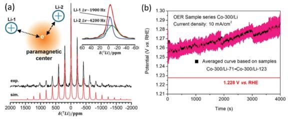
Fig. 92 (a).7Li MAS NMR spectrum of (as-prepared) Co-300/Li recorded at 11.7 T and a MAS frequency of 25.0 kHz, showing a broad, asymmetric spinning sideband pattern characteristic of a strong electron-Li dipolar interaction. (b). Averaged chronopotentiometry curve based on 53 samples of the sample series Co-300/Li (blacksquares) with standard error bars (magenta). Reproduced with permission from ref. 1324. Copyright American Chemical Society 2018.
