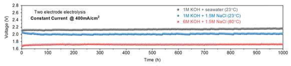
Fig. 153 Durability tests (1000 h) recorded at a constant current of 400 mA cm<sup>-2</sup> of the seawater-splitting electrolyser under 1 M KOH + real seawater at room temperature and 6 M KOH electrolyte at 80 °C, respectively. (h) Reproduced with permission from ref. 1857. Copyright PNAS 2019.
