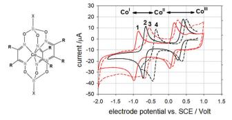
Fig. 107 (a) General chemical formulae of cobalt clathrochelates. (b) Cyclic voltammograms recorded on three different cobalt clathrochelates in acetonitrile (10 mV s<sup>-1</sup>). Complex **1**: X = n-butane and R = cyclohexane; complex 2: X = F and R = methyl group; complex 3: <math>X = n-butane and R = methyl group;phenyl group; complex 4: X = F and R = phenyl group. Reproduced with permission from ref. 1443 Copyright Wiley 2008
