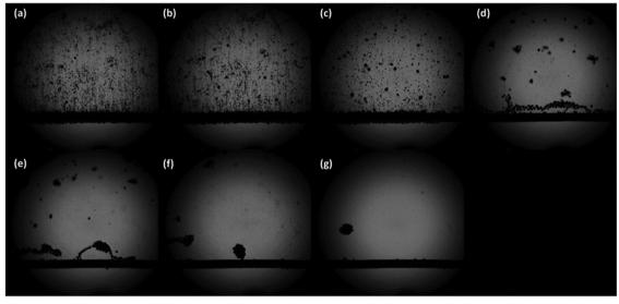
Fig. 149 Hydrogen evolution on a Pt wire in the absence (top left corner) and presence of ultrasound (26 kHz, 100% ultrasonic amplitude). The applied potential was set at -1.30 V vs. RHE - (a) 0  $\mu$ s, (b) 100  $\mu$ s, (c) 200  $\mu$ s, (d) 300  $\mu$ s, (e) 400  $\mu$ s, (f) 500  $\mu$ s, (g) 600  $\mu$ s. The time between each image is  $10^{-4} \text{ s}$ (100 µs) filmed at 10 000 frames per second. Reproduced with permission from ref. 1836. Copyright Elsevier 2020.
