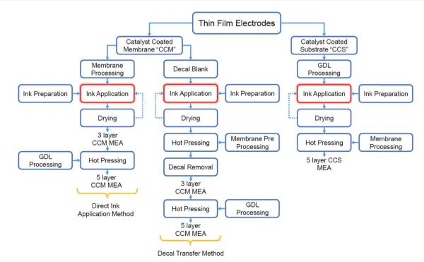
Fig. 108 Overview of multi-steps processes used for CLs, CCMs, and MEAs manufacturing for PEM fuel cells.
