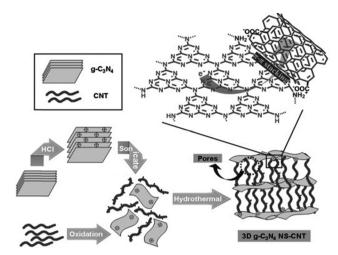
Fig. 100 Fabrication of the 3D q-C3N4 NS-CNT porous composite. Reproduced with permission from ref. 1410. Copyright Wiley 2014.
