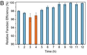
Fig. 152 Cation-selective layer generation during anodic activation (A) chronopotentiometry plot whilst second activation step in salty electrolyte. (B) The associated OER relative faradaic efficiency plots for O<sub>2</sub> production. Reproduced with permission from ref. 1857 Copyright PNAS 2019.
