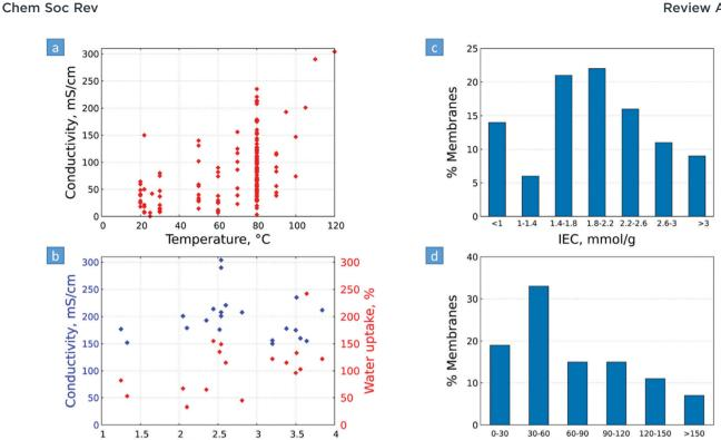
Fig. 10 (a) AEM hydroxide conductivity vs. temperature, and (b) hydroxide conductivity and water uptake of selected AEMs (with conductivities ≥150 mS cm<sup>-1</sup>). (c) Fraction of AEMs at different levels of (c) IEC range and (d) water uptake range. Water uptake values are given in different temperatures. Represented data and the underlying sources are given in Table S1 (ESI†).
