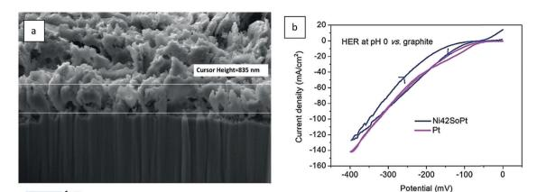
Fig. 106 (a) SEM photograph showing the cross-section of the Ni<sub>42</sub>/Pt interface (Pt thickness ~800-900 nm); the Pt loading is 1.8 mg cm<sup>-2</sup>, (b) comparison of the HER performances of Pt and Ni<sub>42</sub>SoPt at pH = 0. Reproduced with permission from ref. 1269. Copyright Wiley 2019.
