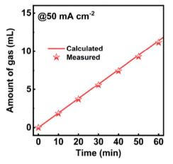
Fig. 154 Theoretically calculated and experimentally measured O2 amounts for NCFPO/C@CC as a function of time in the NaCl + KOH electrolyte. Reproduced with permission from ref. 1858. Copyright ACS
