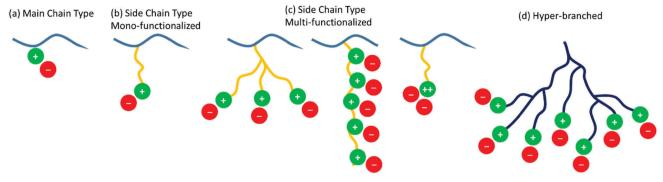
Schematic representation for (a) main chain type, (b) comb-shaped, (c) side chain type with multi-cationic head groups, and (d) hyper-branched **AEMs**
