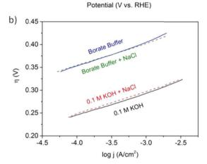
Fig. 151 (a) Electrocatalytic OER activities of NiFe LDH nanoplates supported on carbon, measured using LSV in four different electrolytes after CV "break-in" (50 cycles). A potential of approximately 480 mV, corresponding to the design criteria limit, is marked by a dashed vertical line. (b) Corresponding Tafel plot for low current density j. Measurement conditions: room temperature, 1600 rpm, and scan rate of 1 mV s<sup>-1</sup>. Reproduced with permission from ref. 1864. Copyright Wiley 2016.
