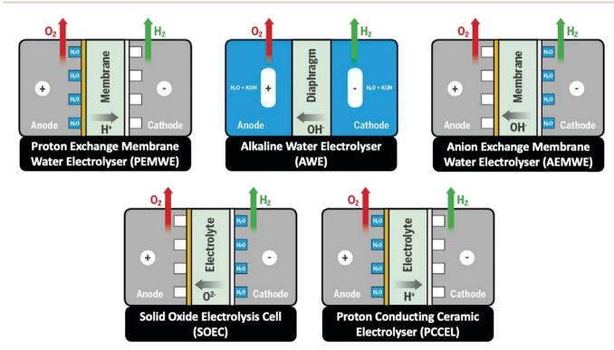
Scheme 3 Schematic presentation of the five main types of water electrolysers.
