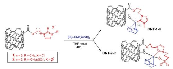
Fig. 125 General Procedure for the Synthesis of Hybrid Carbon Nanotubes-Based Irl-NHC Catalysts. Reprinted with permission from ref. 1552. Copyright 2019. American Chemical Society
