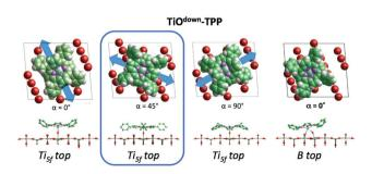
Fig. 22 Side and top views of the equilibrium configurations for different azimuthal orientations of TiO<sup>down</sup>-TPP adsorbed atop a Ti<sub>5f</sub> atom, as well as above the B adatom site, after coordination to an adjacent O<sub>br</sub> atom
