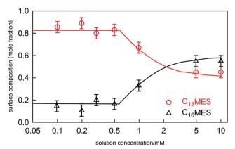
Fig. 10 Variation in surface composition with solution composition for the 65:35 mole ratio eutectic mixture of  $C_{16}MES/C_{18}MES$ . The lines are model calculations using the PPA with the parameters given in the text. Redrawn from Xu et al. 114
