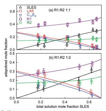
Fig. 18 Variation in adsorbed mole fraction for each component in the quinary mixture, SLES/LAS/C<sub>12</sub>E<sub>8</sub>/R1/R2, containing fixed mole fractions of R1 and R2. Reproduced by permission from Liley et al. 113
