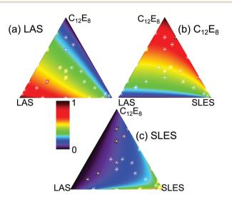
Fig. 17 Composition of the adsorbed layer for the ternary SLES/LAS/C<sub>12</sub>E<sub>8</sub> mixture at a solution concentration of 2 mM. Each triangular diagram, (a)-(c) represents the distribution of the adsorbed fraction of each component using the PPA parameters derived from the binary interactions. The data points are white asterisks on a coloured spot, which disappears when there is exact agreement between experiment and calculation. Redrawn from Liley et al. 112
