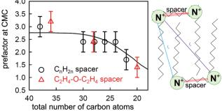
Fig. 8 The experimentally determined prefactor P in the Gibbs equation at the CMC (points) of  $C_nNMe_2C_6NMe_2C_nBr_2$  (black circles) and  $C_nNMe_2C_2-O-C_2NMe_2C_nBr_2$  (red triangles) and a calculated value (line) based on the structure shown alongside and a model described in the text. The two points at 28 carbons have been laterally displaced from each other for clarity. Key distances between charged groups are marked in the structure shown. Figure redrawn from Li et al. 80
