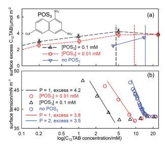
Fig. 5 (a) Surface excesses of  $C_{12}TA^+$  measured by NR at the A–W interface of  $C_{12}TAB$  on its own and with added amounts of 0.01 mM and 0.1 mM POS $_3$  (trianion structure as shown in (a)), (b) the ST of the same set of solutions with fits of the integrated Gibbs equation using the prefactors and the surface excesses at the measured CMC given in the diagram, and the ST at the plateau. Data redrawn from Jiang  $et\ al.^{57}$
