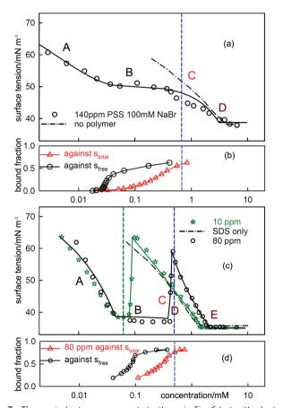
Fig. 7 The equivalent measurements to those in Fig. 6 but with electrolyte, (a) C<sub>12</sub>TAB with NaPSS (MW = 18k) at a concentration of 140 ppm with 100 mM NaBr and (c) SDS with 10 ppm and 80 PDDA (MW = 100k) with 100 mM NaCl. The NR data are redrawn from ref. 69 and 70 and the binding isotherms redrawn from ref. 64 and 65
