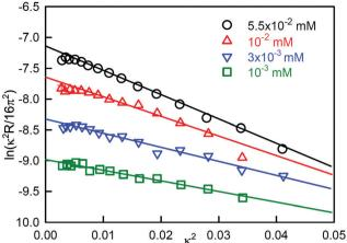
Fig. 1 Linear extrapolation of reflectivity data for C<sub>12</sub>E<sub>3</sub> solutions to obtain the surface excess at various concentrations using eqn (4). Data redrawn from Lu et al.1
