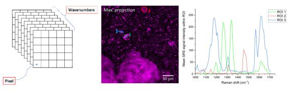
Fig. 8 Hyperspectral SRS imaging schematic (left); maximum intensity projection of a hyperspectral SRS stack acquired by recording SRS images of the sample with 0.1 nm increments in wavelength of the pump beam (middle); resulting SRS spectra generated from the ROIs indicated (right).
