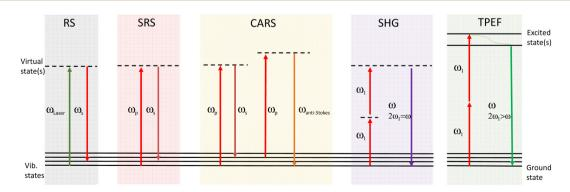
Fig. 2 Jablonski diagrams for spontaneous Raman, SRS, CARS, two photon excited fluorescence, and second harmonic generation, where  $\omega$  is the frequency, and subscript 's' and 'p' indicate the Stokes and pump fields respectively. The green wavy line in TPEF represents relaxation.
