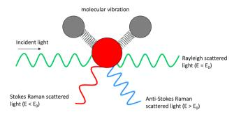
Fig. 1 Raman scattering schematic
