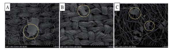
Fig. 9 SEM images of fabrics incorporated with Chinese herb microcapsule: (A) cotton; (B) polyester; (C) nonwoven; this figure is reproduced from the ref. 120 (Gigvvy science open access publishing platform, subject to CC BY-SA 4.0 creative common attribution license).
