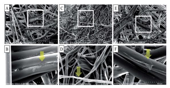
Fig. 10 SEM images: (A and B) first-layer; (C and D) second-layer; (E and F) third-layer of a commercial three-layered surgical mask coated with 1% GS5. (A), (C) and (E) have a magnification of  $150\times$ . White boxes in (A), (C), and (E) is magnified by  $1000\times$ , as shown in (B), (D), and (F). This figure is reproduced from ref. 100 with permission from Taylor & Francis, copyright 2016.
