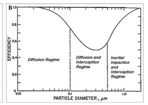
Fig. 3 (A) Particles filtration mechanisms in face masks; (B) face mask filter efficiency *versus* particle diameter. (B) is reproduced from the ref. 53 (open source subjected to creative common attribution 3.0 license).
