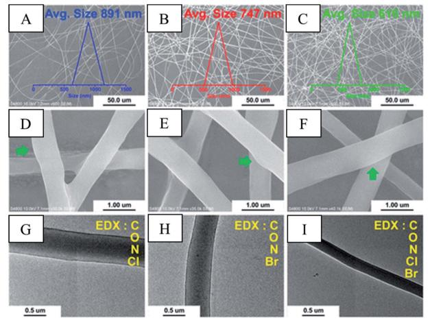
Fig. 11 SEM image: (A and D) PMMA–DCDMH; (B and E) PMMA–DBDMH; (C and F) PMMA–DCDMH/DBDMH; TEM image: (G) PMMA–DCDMH; (H) PMMA–DBDMH; (I) PMMA–DCDMH/DBDMH nanofibres developed through electrospinning. This figure is reproduced from the ref. 229 with permission from American Chemical Society, copyright 2016.
