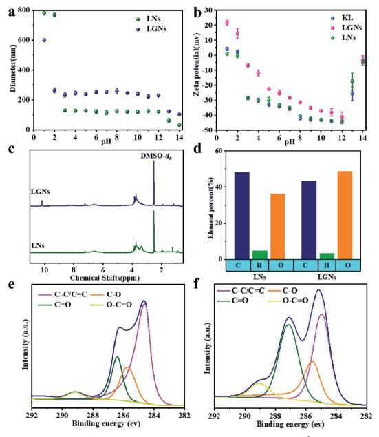
Fig. 2 (a) Zeta potential of particles and (b) average diameter in aqueous media with different pH values. (c) <sup>1</sup>H NMR spectrum of LNs and LGNs. (d) Element contents and (e) C1 XPS peaks of LNs. (f) C1 XPS peaks of LGNs.
