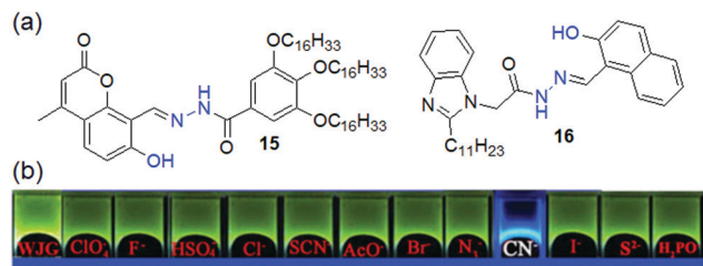
Fig. 13 (a) Structures of compounds 15 and 16 . (b) Fluorescence response of organogel 16 (WJG) to the presence of various anions. Reproduced from ref. 198 with permission from The Royal Society of Chemistry (RSC) on behalf of the Centre National de la Recherche Scientifique (CNRS) and the RSC.
