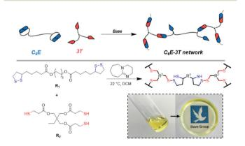
Fig. 1 Schematic illustrating the synthesis of disulfide-based CAN (C<sub>6</sub>E-3T) assuming 1:1 disulfide to thiol. Inset shows photograph of monomer solution and subsequent crosslinking to afford homogeneous film after solvent evaporation.
