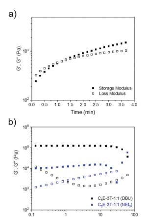
Fig. 2 (a) Rheology time sweep (10% strain, frequency of 1 Hz) at 25 °C to characterise gelation time of  $C_6E-3T-1:1$  using 1 mol% DBU. (b) Frequency sweep analysis showing storage and loss modulus *versus* frequency for networks synthesized using DBU or NEt<sub>3</sub> at 25 °C (1% strain from 0.1 to 10 Hz, or 0.06 to 62 rad s<sup>-1</sup>).
