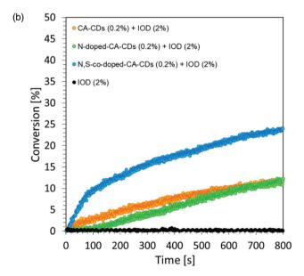
Fig. 10 Free-radical photopolymerization profiles (acrylate function conversion vs. irradiation time) for TMPTA with the bimolecular photo-initiating system based on IOD (2.0 wt%) and CDs (0.2 wt%) (a) under irradiation at 365 nm; (b) under irradiation at 405 nm. Irradiance was measured at a distance of 210 mm for all sources.
