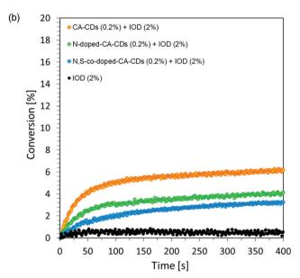
Fig. 7 Cationic photopolymerization profiles (vinyl function conversion vs. irradiation time) initiated by a bimolecular photoinitiating system based on IOD (2.0 wt%) and CDs (0.2 wt%) (a) under irradiation at 365 nm and (b) under irradiation at 405 nm.
