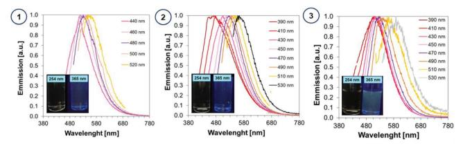
Fig. 6 Fluorescence spectra of aqueous solutions of (1) CA-CDs, (2) N-doped-CA-CDs, and (3) N,S-doped-CA-CDs determined with the use of various excitation wavelengths.
