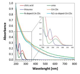
Fig. 5 UV–visible absorption spectra of the synthesized citric acid-based CDs (CA-CDs, N-doped-CA-CDs, N,S-co-doped-CA-CDs) dissolved in water (0.01 g mL<sup>-1</sup>) and the organic molecular precursors for the synthesis of CA-CDs.
