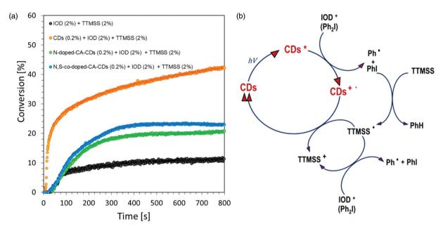
Fig. 9 (a) Cationic photopolymerization profiles (epoxy function conversion vs. irradiation time) initiated by a photoinitiating system based on IOD (2.0 wt%), TTMSS (2.0 wt%) and CDs (0.2 wt%) under irradiation at 405 nm. (b) Schematic cycle of operation of the initiating system consisting of IOD, TTMSS and CDs.
