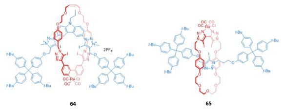
Fig. 38 [2]rotaxanes with a rhenium(1) complex integrated into the macrocycle. 64 binds various halides while 65 binds chloride preferentially with  $K_a = 560 \text{ M}^{-1} \text{ in CHCl}_3.$
