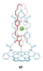
Fig. 40 A hetero-[2]catenane incorporating a zinc porphyrin chromophore which selectively binds  $Cl^{-}$  ( $K_a = 2144 M^{-1}$  in DMSO-d<sub>6</sub>).
