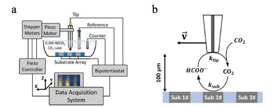
Fig. 4 (a) SECM operation principle; (b) the SG/TC mode all panels reproduced with permission.<sup>128</sup> Copyright 2020, Springer Nature.
