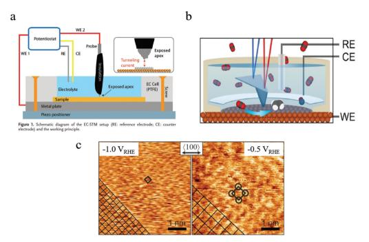
Fig. 5 (a) Schematic of *in situ* EC-STM setup. Copyright 2018, John Wiley and Sons; (b) schematic of *in situ* EC-AFM; (c) morphology of Cu surface at different potentials characterized by *in situ* AFM. Copyright 2020, John Wiley and Sons. All panels reproduced with permission.<sup>139,143</sup>
