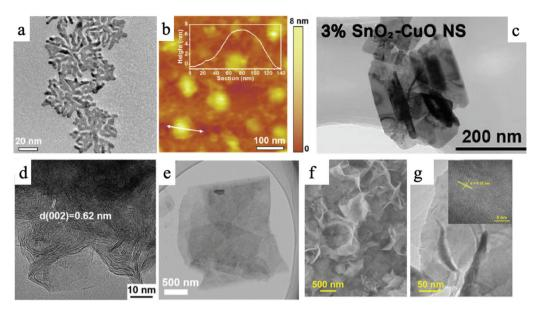
Fig. 1 An overview of different types of 2D materials. (a) and (b) TEM and AFM images of 2D palladium-copper alloy nanodendrites; (c) SnO<sub>2</sub> modified two-dimensional CuO nanosheet; (d) TEM image of MoS<sub>2</sub> nanosheet; (e) TEM image of Ultrathin 2D Mxene. (f) and (g) TEM images of Bi-MOF ultrathin nanosheet. 30-34
