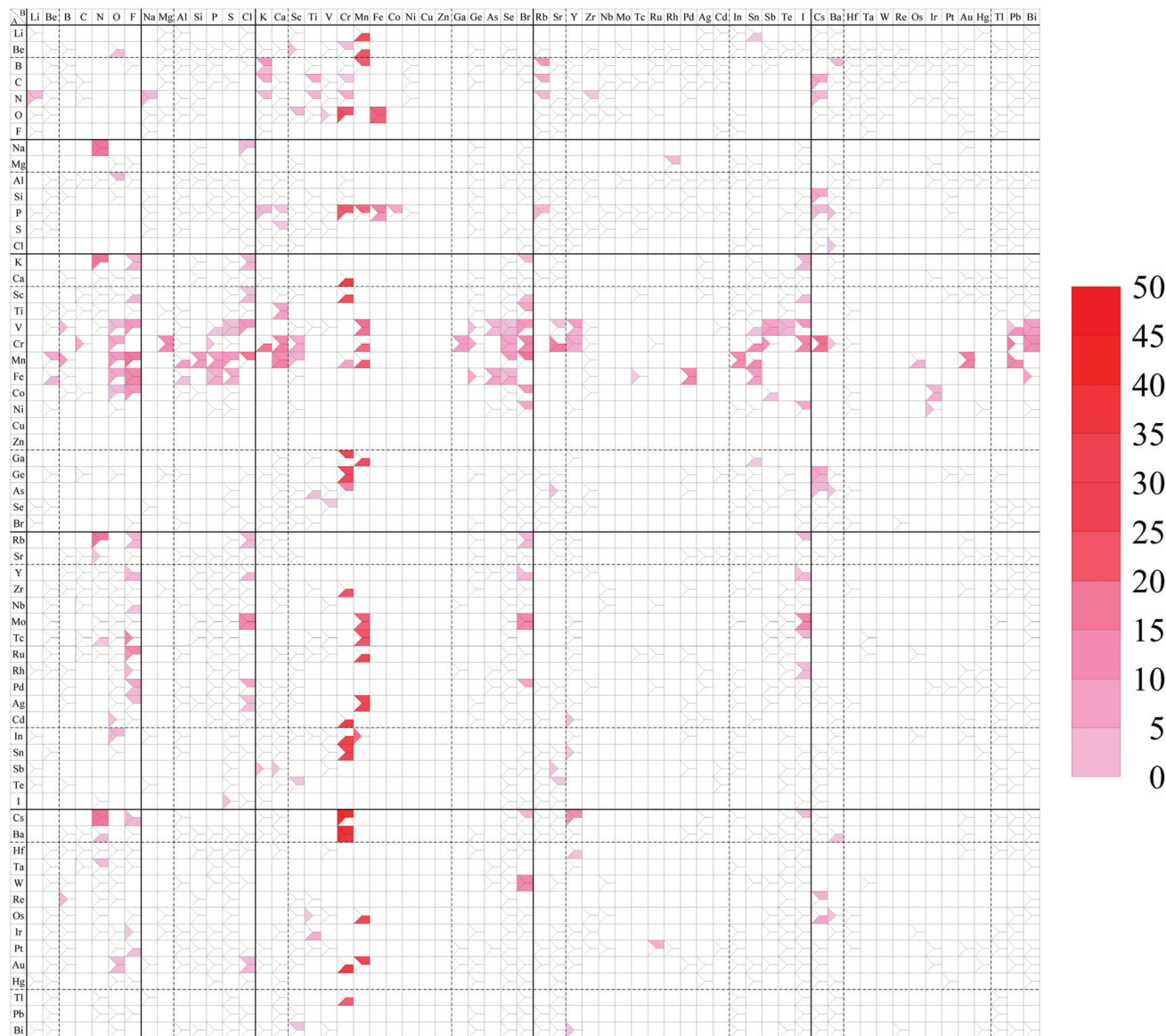
Fig. 11 Spin magnetic moment map for AB_2 type monolayers. The degree of intensity of red color represents the magnitude of the spin magnetic moment [ \mu_B per unit cell].
