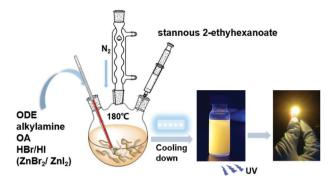
Scheme 1 Schematic diagram of the synthesis of the 2D  $(RNH_3)_2SnX_4$  perovskites by a hot-injection method.
