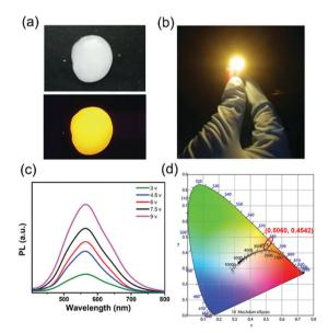
Fig. 5 (a) Images of  $Zn^{2+}$ -doped ( $C_8H_{17}NH_3$ ) $_2SnBr_4$  yellow phosphorembedded in the PS film under sunlight (top) and 365 nm UV light (bottom). (b) 365 nm UV light pumped yellow LED device. (c) PL spectra of a yellow LED obtained by varying the driving voltage. (d) Chromaticity coordinates of  $Zn^{2+}$ -doped ( $C_8H_{17}NH_3$ ) $_2SnBr_4$  yellow phosphor plotted on the CIE1931 chromaticity chart.
