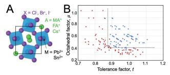
Fig. 1 (A) Perovskite structure comprising corner-sharing octahedra. (B) Plot of octahedral factors versus tolerance factors based on anion-dependent cationic radii. Blue circles represent compounds that form the perovskite structure at room temperature and pressure, while red x's represent those that do not. Adapted from ref. 15. Copyright 2016, Royal Society of Chemistry.
