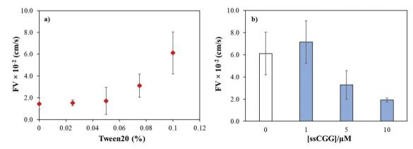
Fig. 2 (a) Effect of surfactant concentration (Tween 20) on flow velocity of PBS buffer (pH 7.4) in wax-on-plastic microchannel. (b) Flow velocity of single-stranded CGG-8 at different concentrations prepared in PBS buffer containing 0.1% Tween 20. Error bar represent standard deviation for three replicates.
