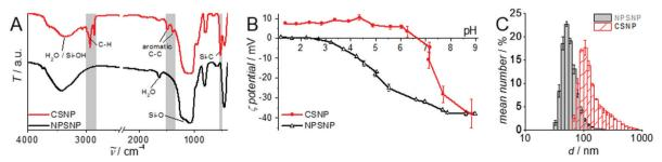
Fig. 1 Characterization of CSNPs (red) in comparison to the core NPSNPs (black). (A) FT-IR spectroscopy; additional bands appearing after the addition of the PMO shell are marked in grey. (B) pH-Dependent zeta potential measurement showing a shift of the isoelectric point after the shell growth. (C) DLS investigations show an increasing particle size comparing the starting material NPSNP (black/grey) and CSNPs (red) equipped with an organosilica shell.
