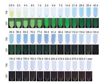
Fig. 7 Supernatants of the release of CSNP\_FCMB starting at 0.5 h up to a sample taken after 1 year. The yellow color and the strong fluorescence under UV light in the beginning show a fast release of FC. A change of color to blue occurs within the first week, afterwards the supernatants are blue and only slightly fluorescent due to the release of most of the FC and the sequential release of MB
