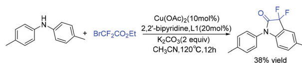
Scheme 101 The copper-catalyzed annulation of N -substituted anilines.
