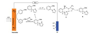
Scheme 8 Possible mechanism of this photo-electrochemical C-H amination.
