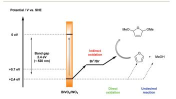
Scheme 6 Plausible mechanism for photoelectrochemical dimethoxylation of furan with Br<sup>+</sup>/Br<sup>-</sup> as a mediator.
