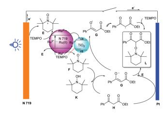
Scheme 12 The plausible mechanism for visible-light-induced α-oxyamination of 1,3-dicarbonyls and TEMPO in PEC cells.
