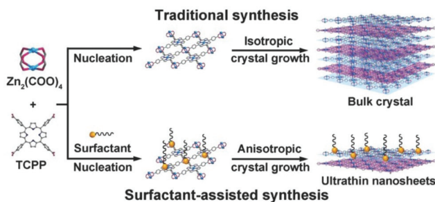
Fig. 12 Preparation of MOFs by traditional synthesis and surfactant-assisted synthesis. In the traditional method, isotropic growth produces large crystals of MOFs, while in the surfactant-assisted synthesis, the surfactant causes anisotropic growth of MOFs to form uniform ultrathin MOF nanosheets. 139 Blue and purple are used to draw MOF layers separately. Copyright, 2015 Wiley-VCH.
