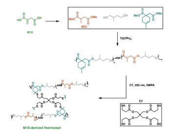
Fig. 16 Cross-linking of M10-derived triblock polymers using C7.93
