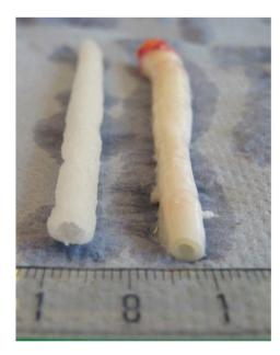
Fig. 15 Porous scaffold (left) synthesised from cross-linked P4 and porcine carotid artery (right).<sup>89</sup> Reprinted from ref. 89, Copyright 2020, with permission from Elsevier.
