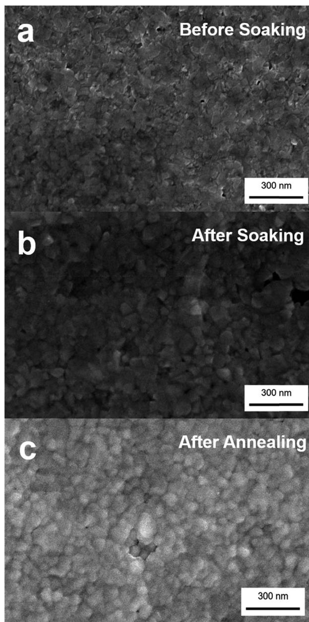
Fig. 2 Scanning electron microscope (SEM) images of (a) Cu<sub>2-x</sub>Se thin film sample before soaking (b) Ag<sub>2</sub>Se thin film after soaking and (c) the Ag<sub>2</sub>Se sample post annealing. The images demonstrate the nano-crystalline grain structure as well as the continuous void-free nature of the Cu<sub>2-x</sub>Se and the Ag<sub>2</sub>Se films. Annealing does not significantly affect the average grain size of the Ag<sub>2</sub>Se film.
