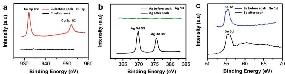
Fig. 4 X-ray photoelectron spectroscopy (XPS) images of (a) Cu peaks at 2p orbital in  $\text{Cu}_{2-x}\text{Se}$  sample before (red) and after (black) soaking, (b) Ag peaks at 3d orbital before (green) and after (black) soaking, (c) Se peaks at 3d orbital before (blue) and after (black) soaking.
