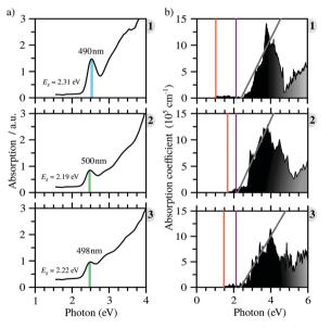
Fig. 3 (a) Experimental absorption data of perovskites 1, 2 and 3, indicating the estimated optical band gap. (b) Theoretical absorption coefficient data of perovskites 1, 2 and 3, indicating the PBE + D3 fundamental band gap as a vertical orange line, the onset of the I p-Bi p transitions as a vertical purple line, and the extrapolation procedure as a gray line, where the point of intersection between this line and the x-axis is the PBE + D3 optical band gap
