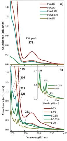
**Fig. 1** UV-Vis spectra of PVA solutions at different concentrations in water (a) before and (b) after ablation. Inset: Comparison of spectra of polyynes solution with and without PVA0.03%. Spectra are obtained after subtraction from the corresponding background spectra, respectively PVA0.03% and PVA0%.
