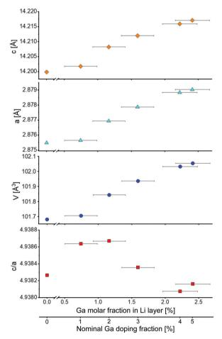
Fig. 3 Lattice parameters a and c, unit cell volume V and c/a ratio as a function of Ga content in the Li layer (as determined by Rietveld refinement). The bottom x-axis indicates the nominal Ga doping. All y-error bars are smaller than the data points
