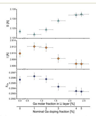
Fig. 4 Layer thickness S, interlayer thickness I and z-coordinate of oxygen  $z_{\rm ox}$  as a function of the Ga content in the Li layer. The bottom x-axis indicates the nominal Ga doping.
