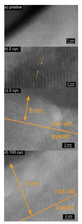
Fig. 7 High-resolution STEM images of Ga-doped LNO (4% nominal doping). (a) Pristine electrode, (b and c) after 2 electrochemical cycles and (d) after 100 cycles.
