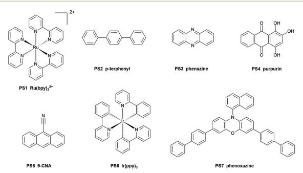
Chart 4 Typical molecular photosensitizers including metal-based (Ru, Ir) complexes and organic aromatic molecules
