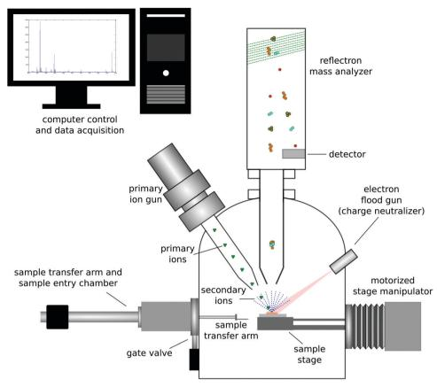
Fig. 3 Schematic drawing of a ToF-SIMS instrument.
