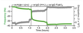
Fig. 11 QCM-D sensorgram showing sequential immobilization of Protein G B1 cysteine mutant (V21C), whole IgG and IgG F(ab')<sub>2</sub> fragment onto a maleimide terminated OEG SAM. The green trace represents the frequency change and the gray trace represents the dissipation change.
