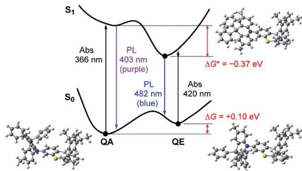
Fig. 5 Schematic energy level diagram for **3** exhibiting the mechanism of excited-state interconversion and dual PL emissions in toluene solution. The optimized structures of the QA and QE conformations in the  $S_0$  state and the orthogonal conformation in the  $S_1$  state calculated at the B3LYP/6-31G(d) level are presented.
