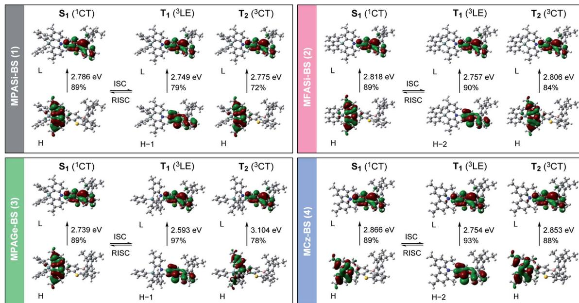
Fig. 7 Electronic transition characteristics and associated frontier orbital distributions for the excited  $S_1$ ,  $T_1$ , and  $T_2$  states of **1–4** calculated using TD-DFT (LC- $\omega$ PBE/6-31+G(d)) at the optimized  $S_1$  or  $T_1$  geometries. The values on each arrow represent the adiabatic excitation energy and contribution weight of the depicted orbitals (H = HOMO; L = LUMO).
