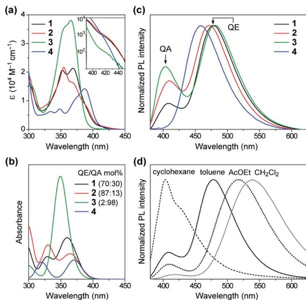
Fig. 4 (a) UV-vis absorption spectra of 1–4 in toluene ( $10^{-5}$  M). The inset shows a magnified view of the lower-energy ICT absorption bands. (b) Theoretical absorption spectra of 1–4 with different populations of QE/QA conformers simulated using TD-DFT (LC- $\omega$ PBE/6-31+G(d)). (c) Steady-state PL spectra of 1–4 in the deoxygenated toluene solutions. (d) Solvatochromic PL responses of 1 in different solvents upon excitation at 350 nm.
