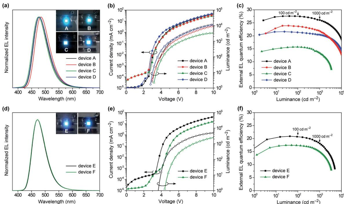
Fig. 8 EL characteristics for (a–c) doped TADF-OLEDs (devices A–D) based on 50 wt% 1–4:PPF and (d–f) non-doped TADF-OLEDs (devices E and F) based on 1 and 3: (a and d) EL spectra measured at  $10 \text{ mA cm}^{-2}$  and photos of blue EL emissions, (b and e)  $J$ - $V$ - $L$  characteristics, and (c and f)  $\eta_{\text{ext}}$  versus  $L$  plots.
