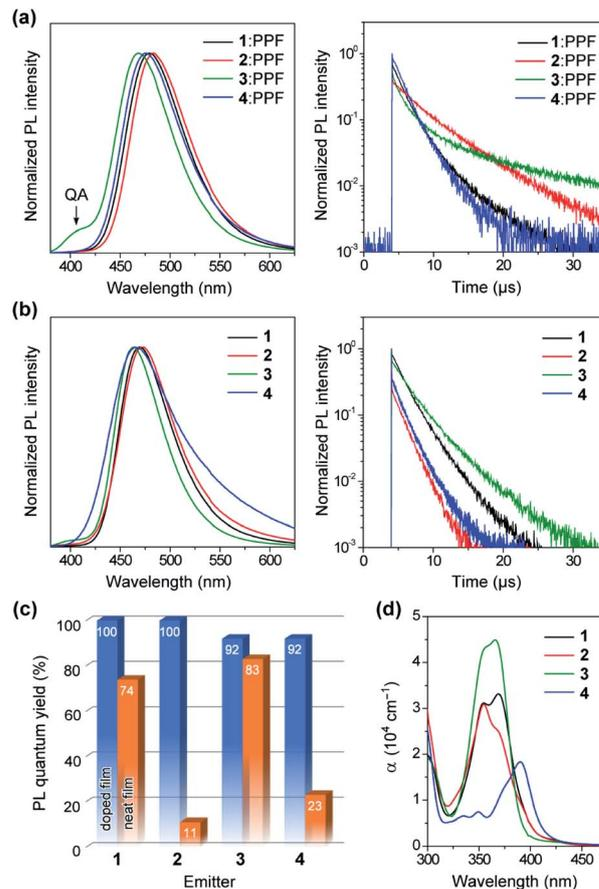
Fig. 6 (a and b) Steady-state PL spectra (left) and transient PL decay profiles (right) of **1–4** in (a) 50 wt%-emitter:PPF doped films and (b) pure neat films measured at 300 K under  $N_2$ . (c) Comparison of  $\Phi_{PL}$  values measured with **1–4** in the doped and neat films. (d) UV-vis absorption spectra of the neat films of **1–4**.
