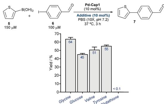
Fig. 3 Pd-Cap<sub>1</sub>-promoted Suzuki–Miyaura reaction of **5** and **6** (top, mean  $\pm$  s.e.m.,  $n = 2$ ), in the presence of additives.
