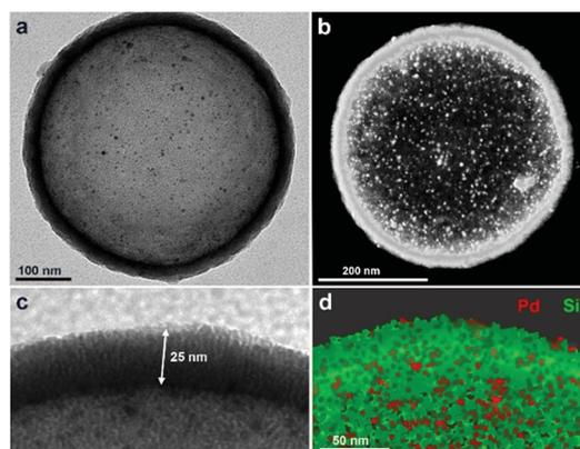
Fig. 2 Characterization of **Pd-Cap1**. (a) Representative TEM image (500 nm diameter); (b) STEM image; (c) zoom-in view showing the vertically oriented mesopores in the silica shell with a thickness of 25 nm; (d) XEDS mapping showing the elemental distribution of Pd and Si.
