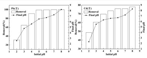
Fig. 5 Effect of pH on adsorption of Pb(II) and Cd(II) on BC/FM. Conditions:  $C_0(Pb(II)) = 100 \text{ mg L}^{-1}$ ,  $C_0(Cd(II)) = 20 \text{ mg L}^{-1}$ , BC/FM dose = 1.25 g L<sup>-1</sup>, temperature = 298 K, and t = 5 h.
