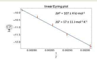
Fig. 4 Eyring analysis for benzyl transfer from [Bn2][Na] to TEMPO.
