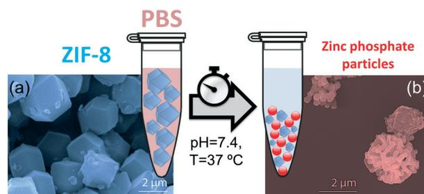
Fig. 1 Incubation process of ZIF-8 particles in phosphate buffered saline media (PBS) under physiological conditions of pH (7.4) and temperature (37  $^{\circ}\text{C}$ ). (a) SEM image of as-synthesized micro-ZIF-8 particles. (b) SEM image of micro-ZIF-8 particles after being soaked in PBS for 24 h.
