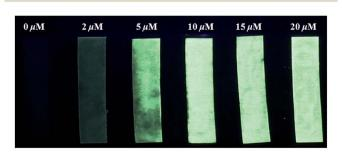
Fig. 8 Fluorescence changes of paper test strips for detecting  $F^-$  in aqueous solution with different  $F^-$  concentrations. The test papers were excited at 365 nm using a hand-held UV lamp.
