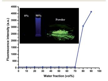
Fig. 1 Fluorescent spectra of HBT (10  $\mu$ M) in the THF/H<sub>2</sub>O mixture at different water fractions,  $\lambda_{ex}=335$  nm,  $\lambda_{em}=470$  nm. Inset: images of HBT (10  $\mu$ M) under UV illumination at 365 nm in THF solution, THF/H<sub>2</sub>O mixture (1 : 9, v/v) and power from left to right.
