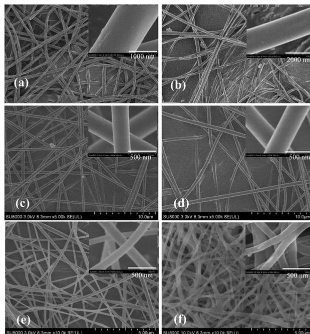
Fig. 3 SEM images of different mass fraction with poly(AN-MA- $\beta$ -CD) in DMF: (a) 36%, (b) 33%, (c) 30%, (d) 25%, (e) 20%, and (f) catalyst bind to poly(AN-MA- $\beta$ -CD).
