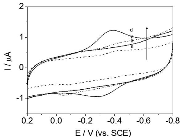
Fig. 7 Cyclic voltammograms of DM-EB/glassy carbon electrode (GCE) (dashed line), Hb/GCE (solid line b), bare electrode (dotted line) and DM-EB/Hb/GCE (solid line d) in PBS at pH 7.0. Scanning rate,  $200 \text{ mV s}^{-1}$ .
