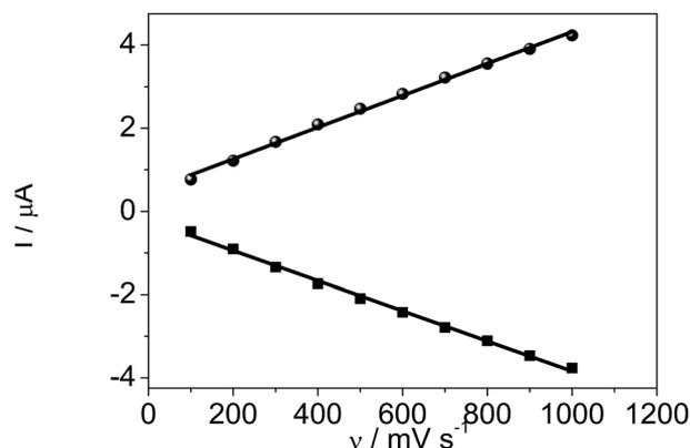
Fig. 8 Plots of oxidation peak current,  $I_{\text{a}}$  (●) and reduction peak current,  $I_{\text{c}}$  (■) vs. scanning rates for DM-EB/Hb/GCE.
