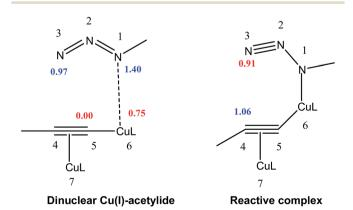
Fig. 3 Local nucleophilicites  $N_{\rm k}$ , (in eV in blue) and local electrophilicites  $\omega_{\rm k}$  (in eV in red) calculated using Parr function.
