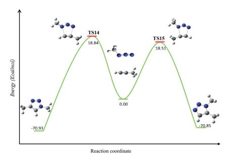
Fig. 4 Calculated energy (kcal mol<sup>-1</sup>) barriers for the uncatalyzed thermal azide–alkyne 32CA reaction in absence of copper(i) species.
