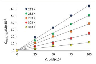
Fig. 4 Variation in the equilibrium concentration of captured  $CO_2$ , plotted as a function of initial FLP (B( $C_6F_5$ )<sub>3</sub> and  $tBu_3P$ ) concentration at T=273 K, 283 K, 293 K, 303 K, and 313 K (repeated in triplicate analysing 300 images with a range of 4000–7000 plugs of  $CO_2$ ) (see ESI† for plots for the other systems).
