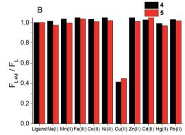
Fig. 5 Fluorescence response of ligands 4 (10  $\mu$ M,  $\lambda_{ex} = 472$  nm,  $\lambda_{em} = 576$  nm) and 5 (10  $\mu$ M,  $\lambda_{ex} = 472$  nm,  $\lambda_{em} = 552$  nm) to an excess (4 equivalents) of selected metal ions in an aqueous sodium cacodylate buffer solution (0.05 M) at (A) pH 7.4 and (B) pH 5.  $F_L$  and  $F_{L+M}$  denote the normalized fluorescence intensity of the free ligand and the ligand in the presence of the metal ion, respectively.
