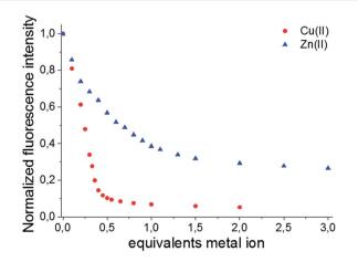
Fig. 4 Fluorescence emission metal titration curve of compound 5 (10  $\mu$ M,  $\lambda_{ex}=472$  nm,  $\lambda_{em}=552$  nm) using Cu(II) (red  $\bullet$ ) and Zn(II) (blue  $\blacktriangle$ ) in an aqueous sodium cacodylate buffer solution (0.05 M, pH 7.4).
