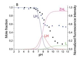
Fig. 3 Fluorescence emission pH titration curves of compound 5 (10  $\mu$ M,  $\lambda_{ex} = 472$  nm,  $\lambda_{em} = 552$  nm) in water in the absence (black  $\blacksquare$ ) or presence of 1 equivalent of metal ion, (A) Cu(II) (red  $\blacksquare$ ) and (B) Zn(II) (blue  $\blacktriangle$ ), and mole fraction distribution diagrams for the various species of this ligand under these conditions (solid lines).
