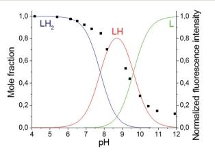
Fig. 2 Fluorescence emission pH titration curve of compound 5 (10  $\mu$ M,  $\lambda_{ex}=472$  nm,  $\lambda_{em}=552$  nm) in water (black  $\blacksquare$ ) and mole fraction distribution diagram for the various protonated species of this ligand (solid lines).
