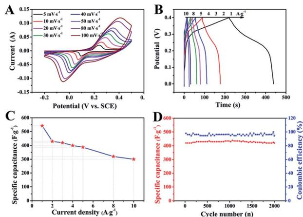
Fig. 5 The electrochemical test results of the  $\text{ZnCo}_2\text{O}_4$  microspheres electrode. (A) The CV curves at various scan rates. (B) The GCD curves at various current density. (C) The capacitance as a function of current density. (D) The cycling performance and Coulomb efficiency at  $2 \text{ A g}^{-1}$ .
