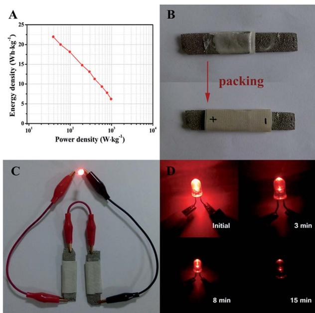
Fig. 7 (A) Ragone plots of the  $\text{ZnCo}_2\text{O}_4//\text{AC}$  quasi-solid-state asymmetric supercapacitor. (B) Digital photographs of the  $\text{ZnCo}_2\text{O}_4//\text{AC}$  quasi-solid-state asymmetric supercapacitor before and after packing. (C) Optical images of a red LED powered by two solid-state asymmetric supercapacitors connected in a series. (D) The evaluation of the lightened red LED at different stages after corresponding to (C).
