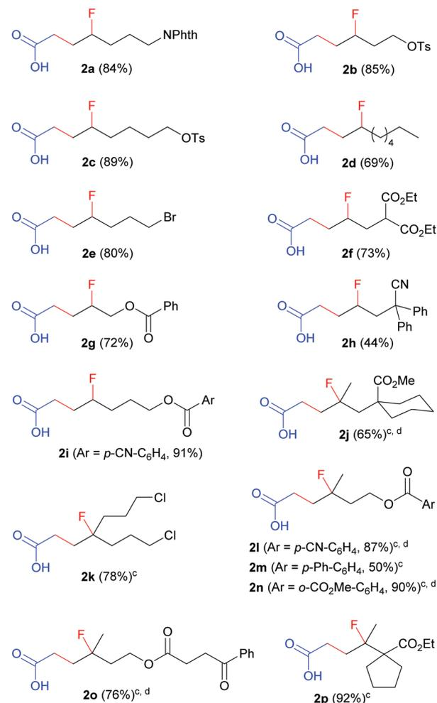
**Scheme 1** Carbofluorination of unactivated alkenes. <sup>a</sup> Reaction conditions: **1** (0.2 mmol), Selectfluor (0.6 mmol), AgNO<sub>3</sub> (0.04 mmol), DCM (0.5 mL), H<sub>2</sub>O (1 mL), AcOH (0.5 mL), H<sub>3</sub>PO<sub>4</sub> (0.8 mL), 50 °C, 24 h. <sup>b</sup> Isolated yield based on **1**. <sup>c</sup> Selectfluor (0.4 mmol) and H<sub>3</sub>PO<sub>4</sub> (0.4 mL) were used. <sup>d</sup> Reaction time: 12 h.
