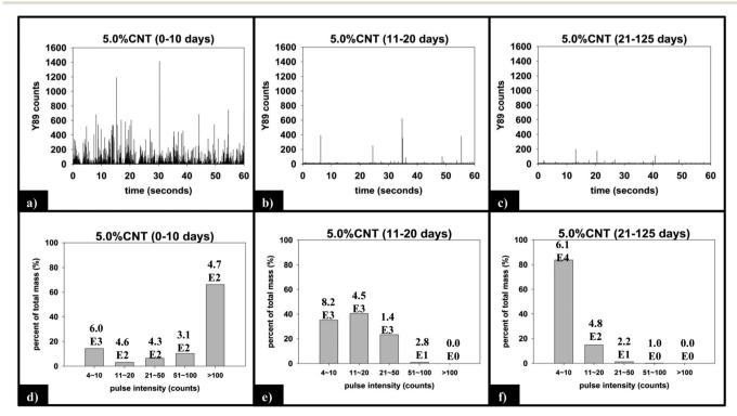
Fig. 8 (a)–(c) Raw sp-ICP-MS data collected for 5.0% CNT nanocomposites with increasing duration of UVC exposure. (d)–(f) Y mass distribution for each period of exposure, with the corresponding number of particles detected noted above each bin.
