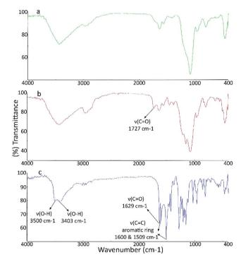
Fig. 1 FT-IR spectra of LMSN-COOH@CS-FA (a), LMSN-COOH-CUR@CS-FA (b) and CUR (c).
